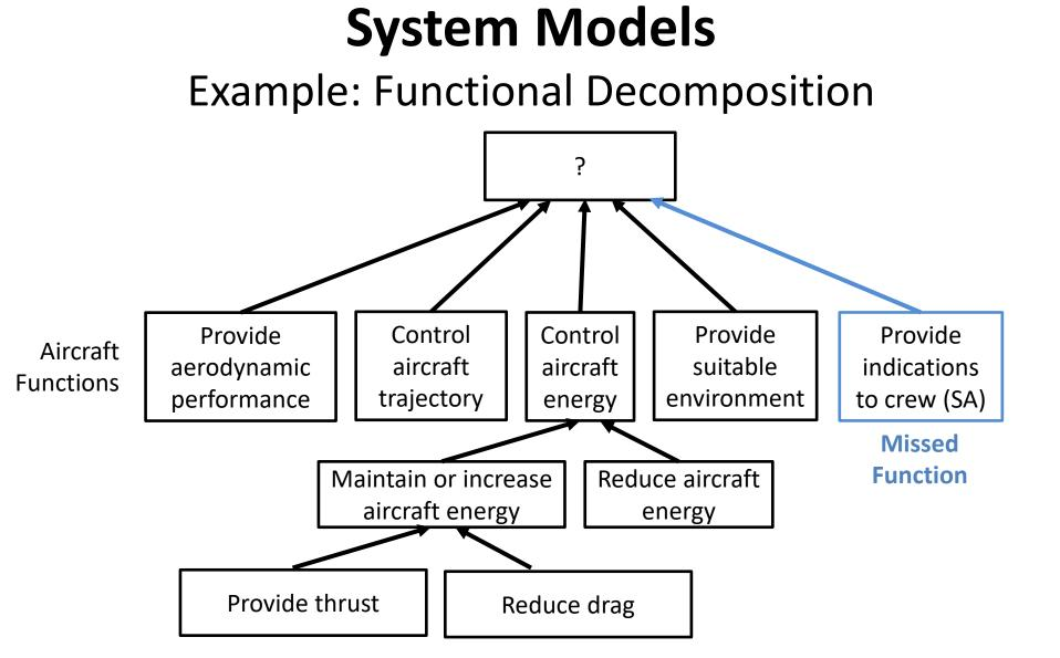
Doesn't help identify missing functions that are needed or functions that may be unsafe as designed
