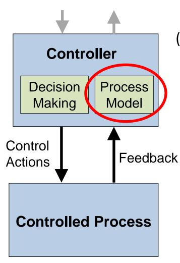
**Model Condition**: The controller must have (or contain) a model of the system
