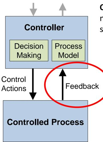
**Observability Condition**: The controller must be able to ascertain the relevant states of the system.
