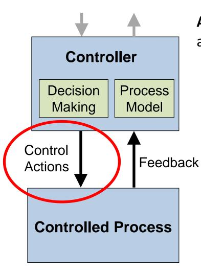
Action Condition: The controller must be able to affect the system state
