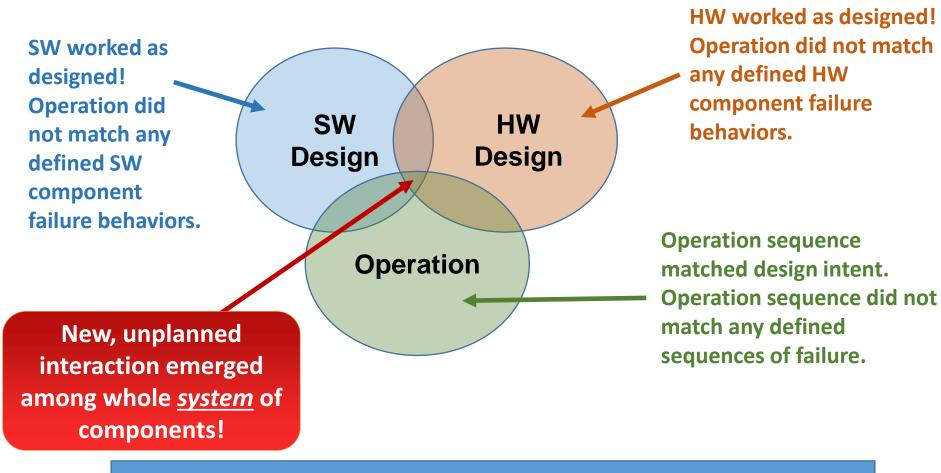
Easy to overlook the <u>system</u> problem by looking at <u>individual component failures</u>
