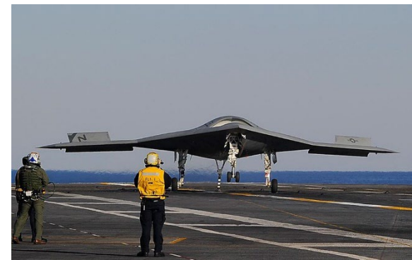
E.g., X-47B UAV integrated into carrier operations alongside manned aircraft. Provides autonomous launch, flight, follow manned A/C, carrier landing, etc.
