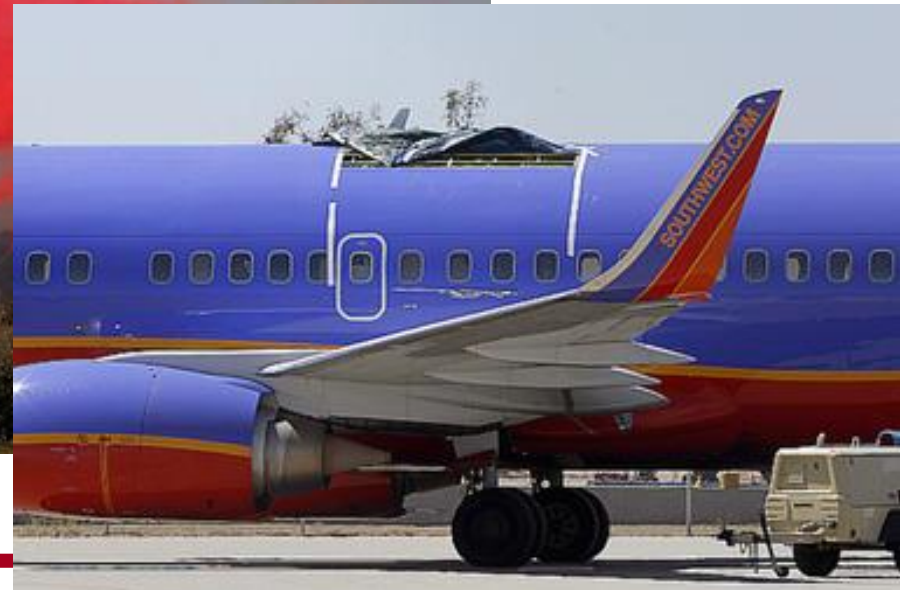
“FAA orders airlines to inspect 737s for cracks: three days earlier, undetected cracks widened into a five-foot hole in the roof of a Southwest 737, forcing an emergency landing”
