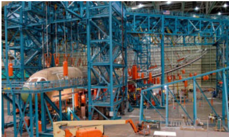
Full scale wing testing. Photo Boeing
