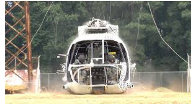
Helicopter crash testing. Photo United States Navy
