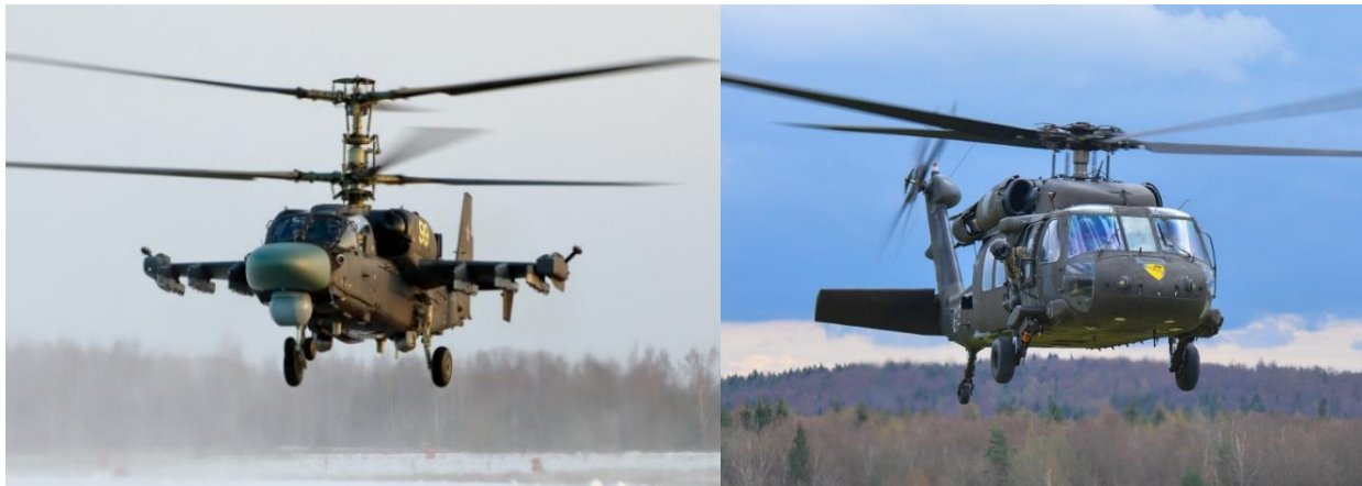
Figure 4-3: Coaxial Helicopter on Left, Single Main Rotor with Tail Rotor Configuration on Right
