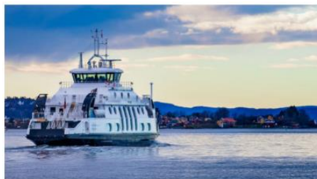
ELECTRIC LOCAL FERRY. Several million people travel emissions-free between Oslo and Nesodden each year. Ferries charge batteries at the pier in front of the town hall. Photo: Geir Anders Rybakken Ørslon
