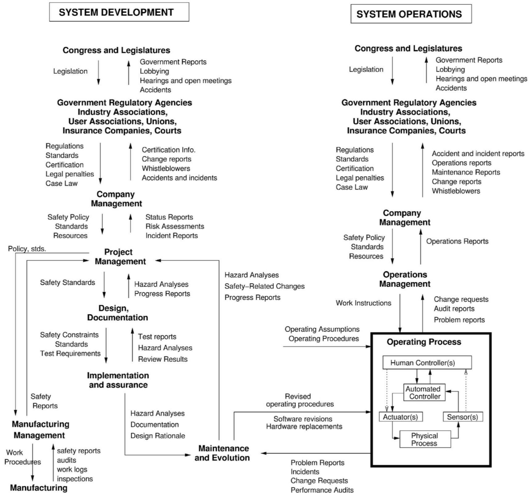
Fig. 7. A generic hierarchical safety control structure.
