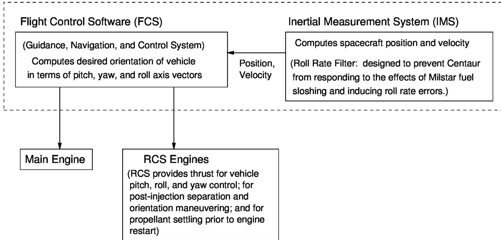
Safety constraint on FCS violated: The FCS must provide the attitude control, separation, and orientation commands to the main engines and RCS to attain geosynchronous orbit
