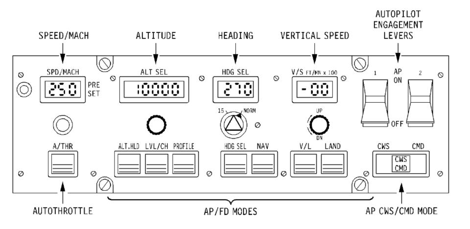
About 7 seconds after the first officer completed the Before Landing checklist, the first officer noted that the captain had switched the autopilot to vertical speed mode; shortly thereafter, the captain increased the vertical descent rate to 1500 fpm.
