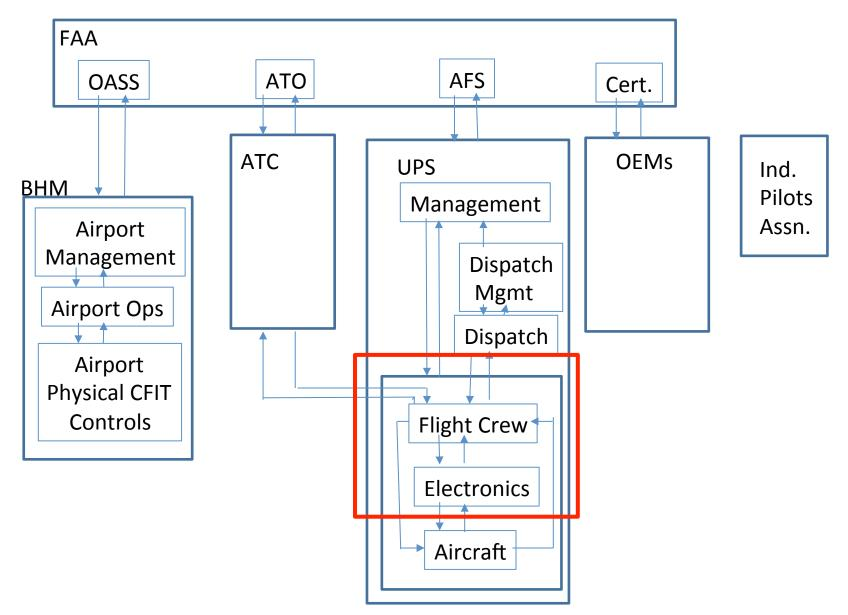
**Unsafe Control Action**: Did not properly configure (program) the FMC for a profile approach. Did not call for pilot monitoring to verify the flight plan in the FMS.
