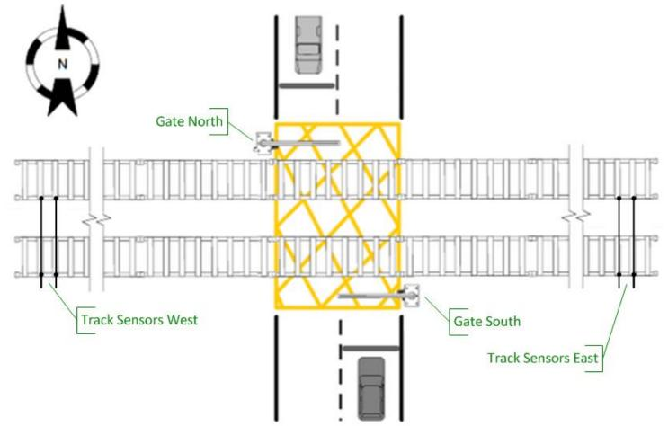
Illustration adapted from Y.S. Weng, et al., Design of Traffic Safety Control Systems for Railroads and Roadways Using Timed Petri Nets
