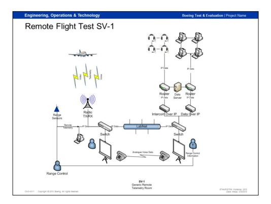
LabNet is a Boeing wide VPN providing high bandwidth, low latency network communication.
