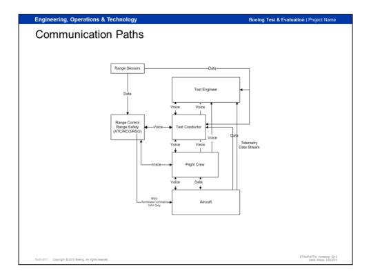
The overall communication paths are straight forward. Voice is communicated to the flight crew, and voice and data are returned. The external range sensors can range from the simple to complex, however in all cases the data is provided digitally to the test team an range control team.
