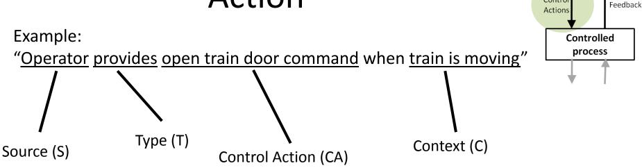
Four parts of a hazardous control action
