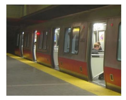
System Hazards H-1: Doors close on a person in the doorway H-2: Doors open when the train is moving or not at platform H-3: Passengers/staff are unable to exit during an emergency
